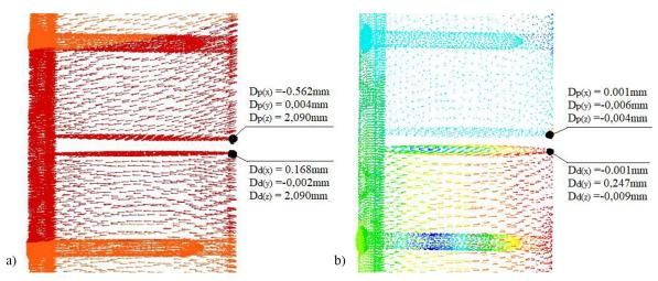
Figure 7. Point displacement vectors for the case of a Broad DCP: a) axial load, b) torque
