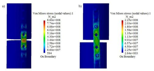
Figure 5. Von Mises stress on a Narrow LC-DCP: (a) axial load, (b) torque
