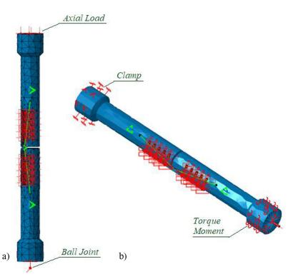
Figure 4. Defining constraints and loads: (a) axial load, (b) torque
