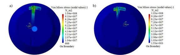
Figure 6. Von Mises stress on the cross-section of the most loaded bolt of a Broad DCP: (a) axial load, (b) torque
